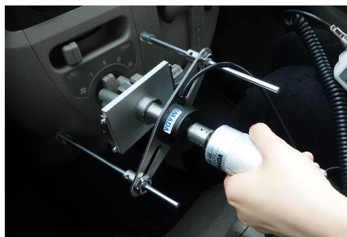
For feeling test of rotary switches on car dashboard
